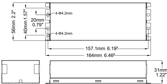
**8W Battery case-** 6.1"x1.2"x1.18"(155mmx30.5mmx30mm)
