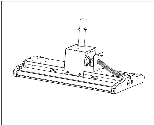
4. Install the two side-covers of the bracket with screws to hide the wires.
