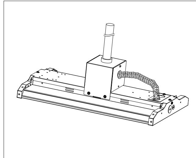
Note : If the outlet board located under the pendant box, do wiring connection directly in the box and no need to use the flexible protective conduit. All wire connectors or terminal caps should be left inside the pendant box.
